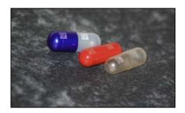
Innomech is developing technologies to print or laser etch two-dimensional dot matrix identifier codes onto a variety of healthcare products. The image above shows a 2 mm x 2 mm matrix code printed onto the surface of drug capsules.
