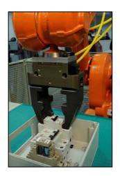
RoBox is essentially a general purpose machine tool that is perfect for multiple manufacturing tasks, such as control hardware assembly as shown here.
