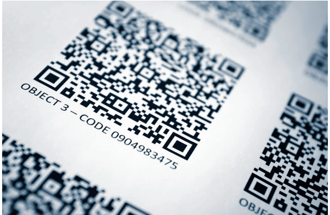
Datamatrix 2D codes have error detection and correction built in
