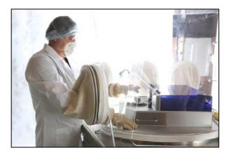
1 Capsugel, Innomech and Powder Systems have worked together to develop Xceloprotect, a novel glove box solution for Xcelodose. Xceloprotect has been designed to further increase operator safety when filling capsules with high potency pharmaceutical powders. Credit: Powder Systems Ltd
