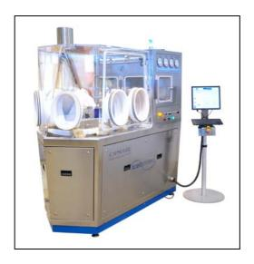
Innomech has re-engineered Xcelodose for easier cleaning, maintenance and to enable integration into a high performance containment system. All the mechanical and electrical mechanisms for the capsule-filling and weighing system have been re-positioned into the lower half of the isolator to avoid contamination and to provide safe and easy access for servicing.
