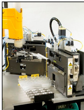
Fig 1 - Tile assembly starts with rows of optical light guides being thermoformed in the 'bending station'.
