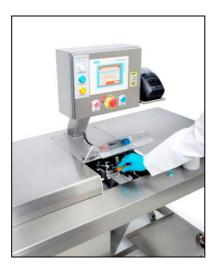
Innomech was appointed by a California-based biotech group to design and build two end-of-line testing systems for a new multi-dose, dial-a-dose drug delivery pen. The easy-to-use system requires minimal operator training to check and record over 20 parameters on the assembled pen.
