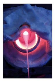
GB Innomech's high-throughput inspection system will enable Cera Dynamics to increase its output of glass frit four-fold. The powders are produced from highly-specified molten glass compositions – shown above being poured from a furnace – which are then solidified, shattered and ground to customised particle sizes. Photo credit: © Exesios Photography
