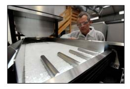
Automation consultancy GB Innomech is developing a high-throughput inspection system for glass frit or powder that will enable specialist glass manufacturer Cera Dynamics to increase its output by 300%.
