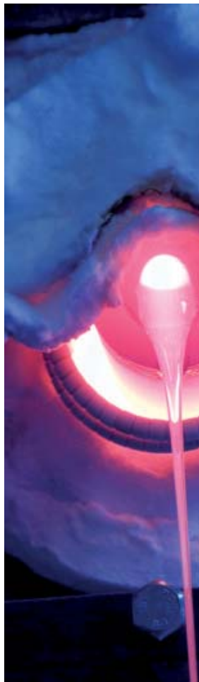
The powders are produced from molten glass compositions – shown above being poured from a furnace – which are then solidified, shattered and ground to customised particle sizes
