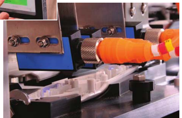
Above: specifications need to evolve. In this example, an extra UV glue checking step was found to be essential in the automated process
