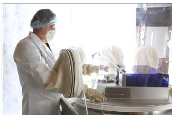
1 Capsugel, Innomech and Powder Systems have worked together to develop Xceloprotect, a novel glove box solution for Xcelodose. Xceloprotect has been designed to further increase operator safety when filling capsules with high potency pharmaceutical powders.
